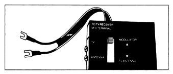
TV/MODULATOR SWITCH That's all there is to it. Turn on your television set and computer, and you're ready to start. Adjust the controls (including "fine tuning") of the television set for optimal picture clarity and most pleasing colors, just as you would for normal television reception.
